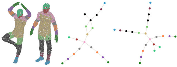
Figure 7: Region-based correspondence between shapes with non-isomorphic shape graphs with different topology. The shape graph of the left shape (shown in centre) contains a loop while the shape graph of the right shape (shown right) has a tree structure.
